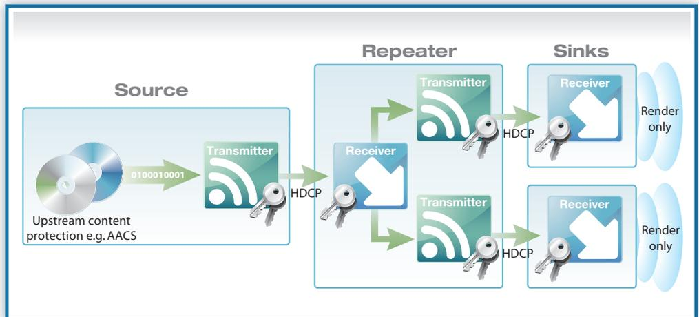
Each HDCP transmitter or receiver includes 40 56-bit secret keys, known as Device Private Keys, as shown in figure 3. These keys, provided by DCP, are unique to the transmitter or receiver, highly confidential and not available to other devices.
